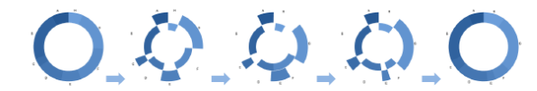
Figure 3. A multi-stage animation of changing values in a donut chart. Stage 1: Wedges split into two rings. Stage 2: Wedges translate to be centered on their final position. Stage 3: Wedges then update their values, changing size. Stage 4: Wedges reunite into a single ring.
